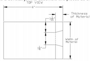
The angle for the Pins and Talls of the dovetall joint is 70-80 degrees.
